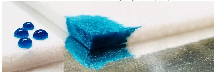
The optional heated liquid inlet is a powerful additional feature for introducing liquid monomers to achieve functional coatings on a wide range of materials. Plasma coatings are uniform, durable and can be applied on any sample geometry to produce a wide range of properties including hydrophilic, hydrophobic and oleophobic surfaces, biocompatible chemistries and biomolecule immobilisation.
